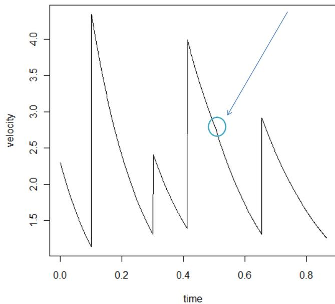
Figure 1: A typical path of the velocity  $v(t)$  is a piece-wise continuous function between two nearest deaths of the contacts. The velocity has jumps at moments of the death of particle. The derivative of the velocity increases abruptly at the moment of the birth of a particle (blue circle).
