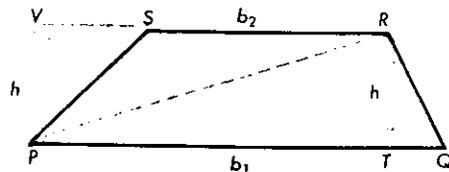
$$A = \frac{1}{2}b_1h + \frac{1}{2}b_2h \\ = \frac{1}{2}h(b_1 + b_2),$$
