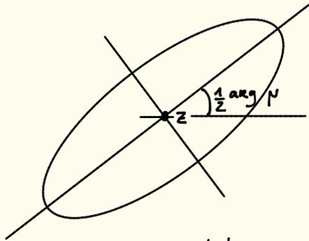
$$\frac{\text{big axis}(z)}{\text{small axis}(z)} = \frac{1+|\mu|}{1-|\mu|}$$
