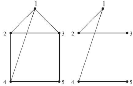
Figure 2. A Graph  $G$  and its Spanning Tree  $T$ .
