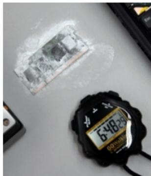
Aplicando um *Canned air* ( $-50^{\circ}\text{C}$ )
