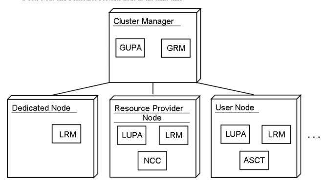
Figure 1: InteGrade's Intra-Cluster Architecture
