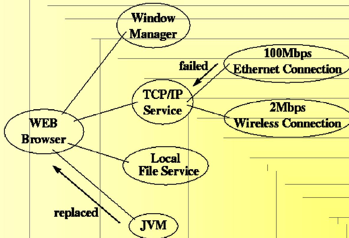
A WEB Browser ComponentConfigurator and its relations to system ComponentConfigurators
