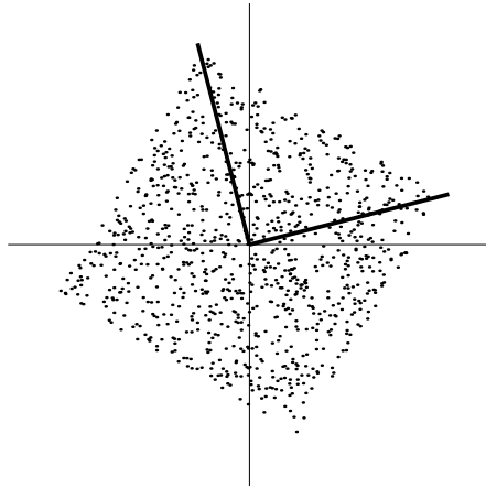
Fig. 9.2 Problems of convergence with the (natural) gradient method for maximum likelihood estimation. The data was two whitened mixtures of subgaussian independent components. The nonlinearity was the one in (9.18), which was not correct in this case. The resulting estimates of the columns of the whitened mixing matrix are shown in the figure: they are not aligned with the edges of the square, as they should be.
