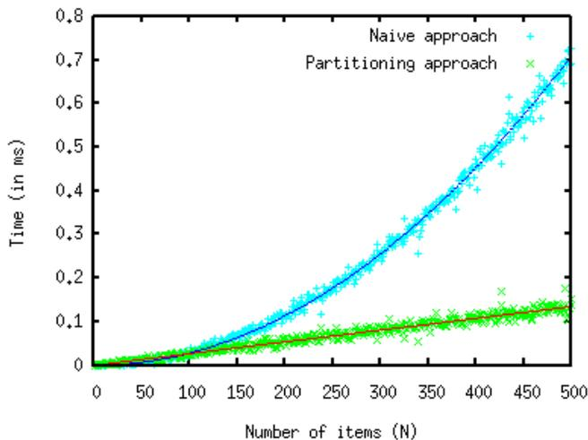
Figure 6: Practical performance of the naive and the partitioning approaches for the overlapping evaluation of an increasing number of randomly distributed identical items.
