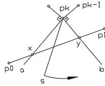
Figure 17: The scan line  $s$  does not hit vertices visible from  $p_k$  as it rotates from  $a$  to  $b$ .
