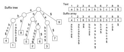
Fig. 1. An example of the suffix tree and the suffix array.
