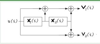
A physical realization for the encoder  $G(D)=\begin{pmatrix} 1+D+D^2 & 1+D^2 \end{pmatrix}$ . This encoder has degree 2 and memory 2.
