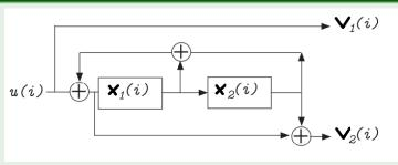
A physical realization for an equivalent encoder G'(D). This encoder has degree 2 and infinite memory.
