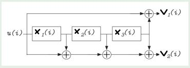
A physical realization for the (catastrophic) equivalent encoder  $G''(D) = (1+D)G(D) = (1+D^3) + D + D^2 + D^3$ . This encoder has degree 3 and memory 3.
