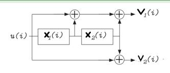
A physical realization for the encoder  $G(D) = (1 + D + D^2 \ 1 + D^2)$ . This encoder has degree 2 and memory 2.
