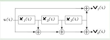
A physical realization for the (catastrophic) equivalent encoder  $G''(D)=(1+D)G(D)=\left(\begin{array}{cc} 1+D^3 & 1+D+D^2+D^3 \end{array}\right)$ . This encoder has degree 3 and memory 3.
