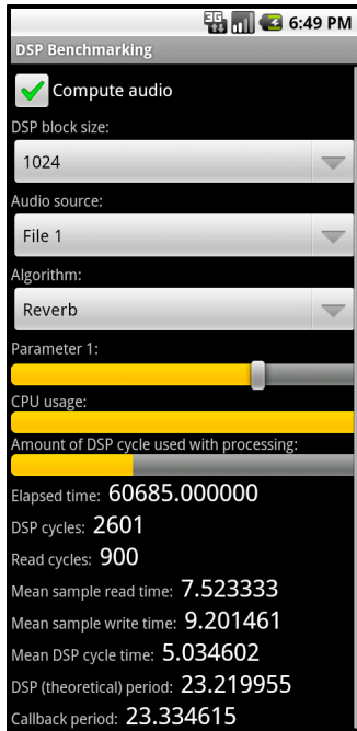
Figure 2. The GUI controlling a live DSP process. The user is able to choose the DSP block size, the audio source (microphone or predefined WAV files) and the DSP algorithm that will be run. Also, slider widgets can provide explicit parameter input, while visual and numerical statistics give feedback about the state of the system.
