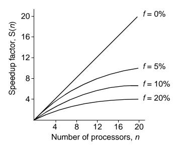
Even with infinite number of processors, maximum speedup limited to 1/f.
