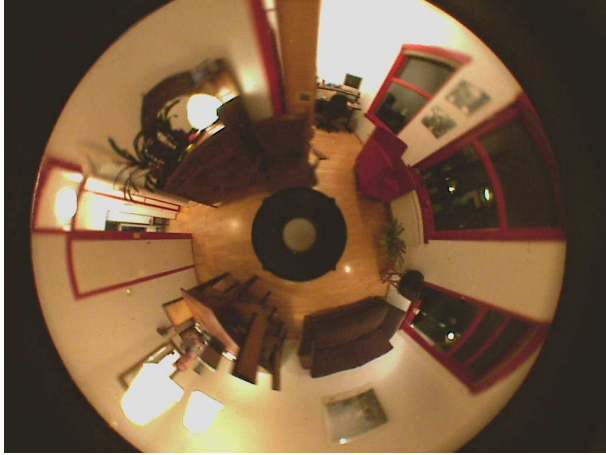
Figure 1. Image obtained from an omnidirectional vision system
