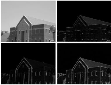
FIGURE 10.11 Same sequence as in Fig. 10.10, but with the original image smoothed with a 5 \times 5 averaging filter.
