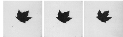
FIGURE 10.43 (a) Original image, (b) Result of split and merge procedure, (c) Result of thresholding (a).
