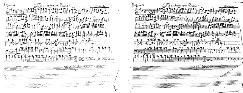
(a) Niblack without histogram equalization (b) Niblack after histogram equalization
